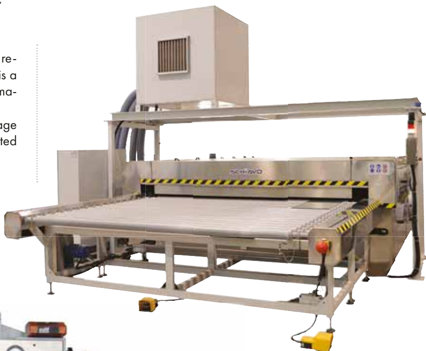
Horizontal glass washing machine HTL2600
