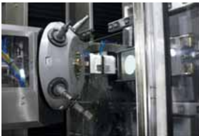
DOUBLE SIDED DRILLING BY 6-SLOTS
