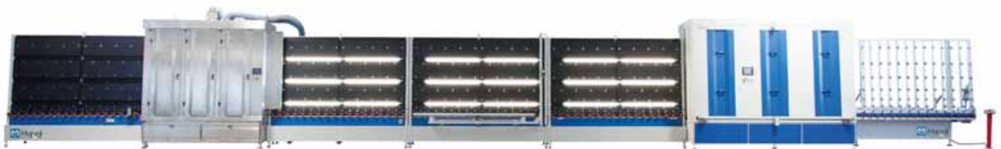
Automatic insulating glass line
